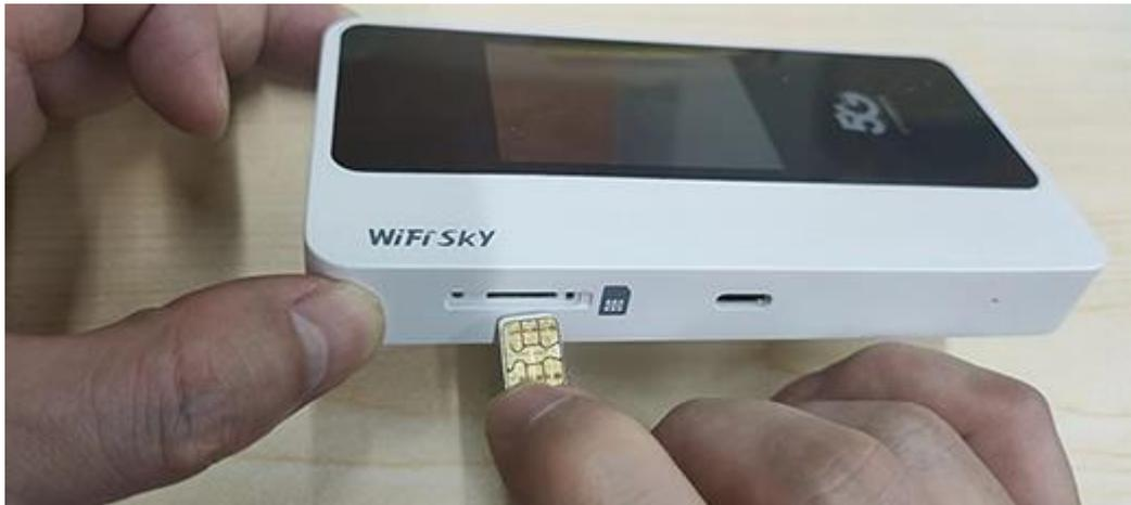
Insert the SIM card into the slot.
