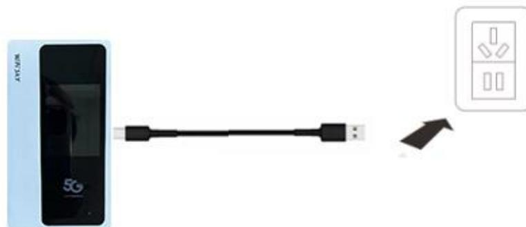
2. Charging the battery by using the USB-A of computer or laptop.
